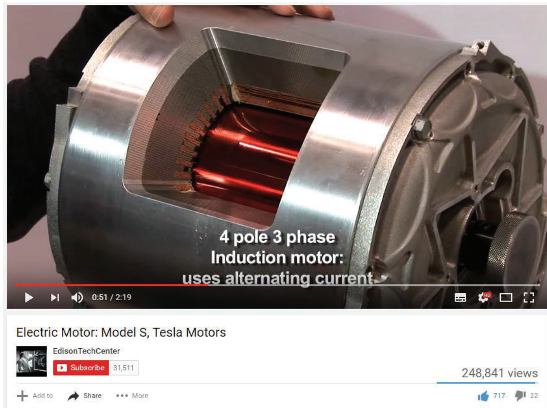
Figure 72 Partial cross section of Tesla Model S' AC induction motor
